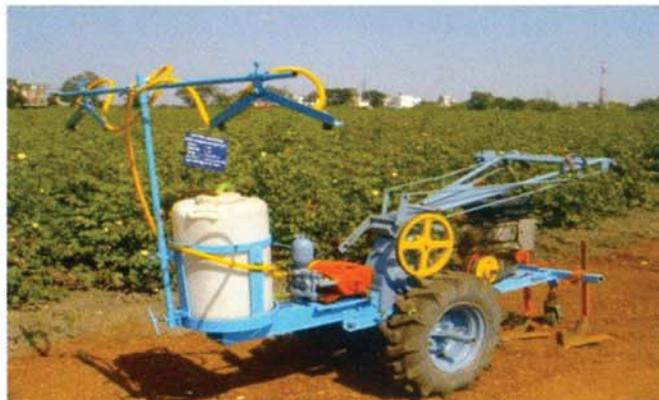
Fig. 2.3.4: view of self propelled weeder cum sprayer
