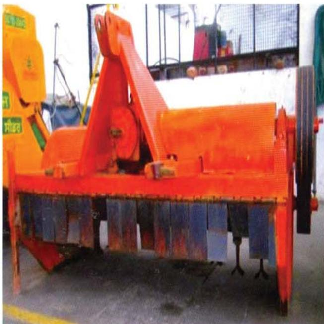
Fig. 2.3.4: A stationary view of tractor operated paddy straw chopper
