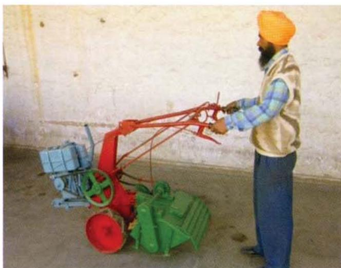
Fig. 2.3.1 : Stationary view of single row manually operated self propelled weeder
