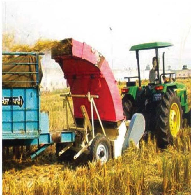
Fig. 2.3.5 :A view of Flail type chopper cum loader for paddy straw cutting and loading
