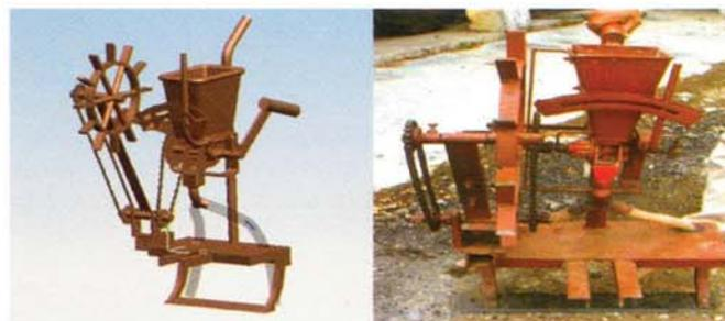
Fig. 2.3.3: Fertiliser applicator attachment with Bakhar
